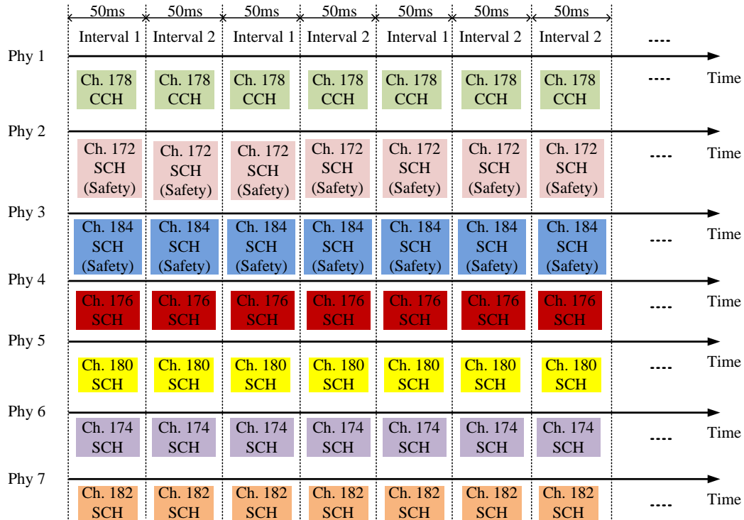
Fig. 7. WAVE multi-channel allocation for seven physical modules
